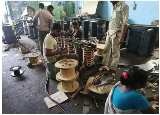
Core and Coil Assembly Section in Sakthi Transformers
