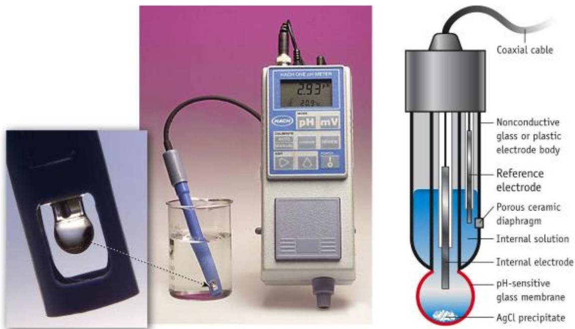
Figure 1. pH meter and a schematic diagram of a glass electrode.
