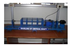
In the construction of whirling of shaft, the following basic features should be considered. The apparatus basically consist of rectangular bed mounted over the rectangular channel. Then three rectangular block of same size is fixed in the bed. The two blocks are fixing in one side and other one is fixed in opposite side.
