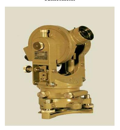
A Tacheometer is used in surveying to determine vertical and horizontal angles by combining optical plummets (or plumb bobs), a spirit (bubble level), and graduated circles. An optical plummet ensures that the theodolite is positioned as vertically above the survey point as possible. The device's internal spirit level ensures that it is parallel to the horizon. The graduated circles, one vertical and one horizontal, enable the user to conduct an actual angle survey.
