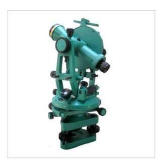
A theodolite works by combining optical plummets (or plumb bobs), a spirit (bubble level), and graduated circles to find vertical and horizontal angles in surveying. An optical plummet ensures the theodolite is placed as close to exactly vertical above the survey point. The internal spirit level makes sure the device is level to to the horizon. The graduated circles, one vertical and one horizontal, allow the user to actually survey for angles.
